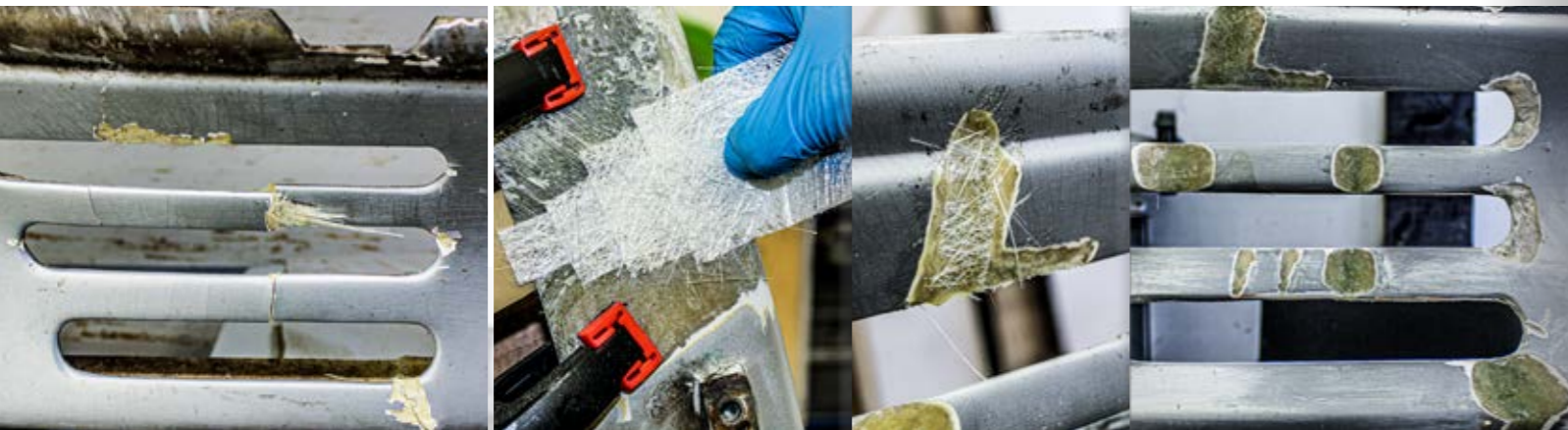
Damaged fiberglass component
