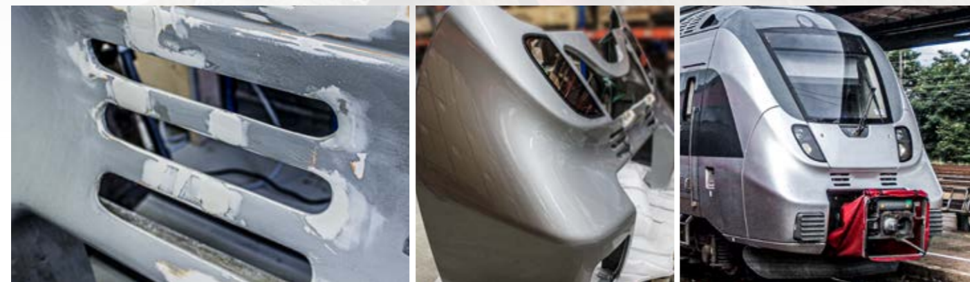
Filled and Restored Surface
